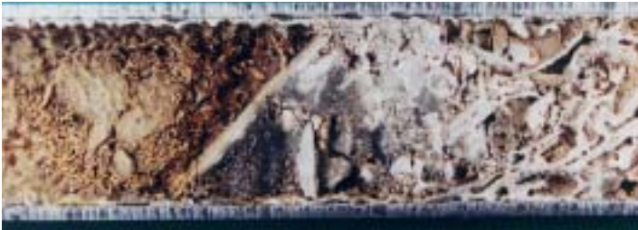
Scaling (Photo: CEBTP)
