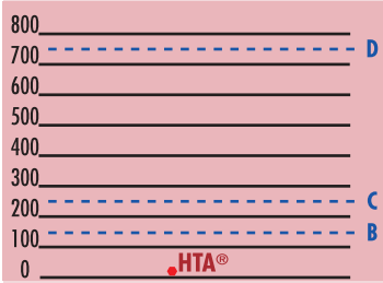
FIGRA w/s (watts/second) the HTA ® index obtained is 2 (which is 1.7% of the max. B)
